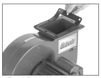
Figure 9. Placing rubber gasket over outlet.
